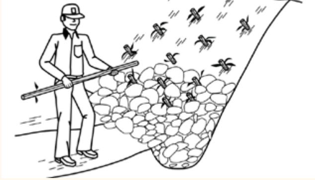
A boulder toe can be added to riparian plantings in high-risk areas where additional bank movement is unacceptable | Illustration by United States Department of Agriculture (USDA) Natural Resources Conservation Service (NRCS)
