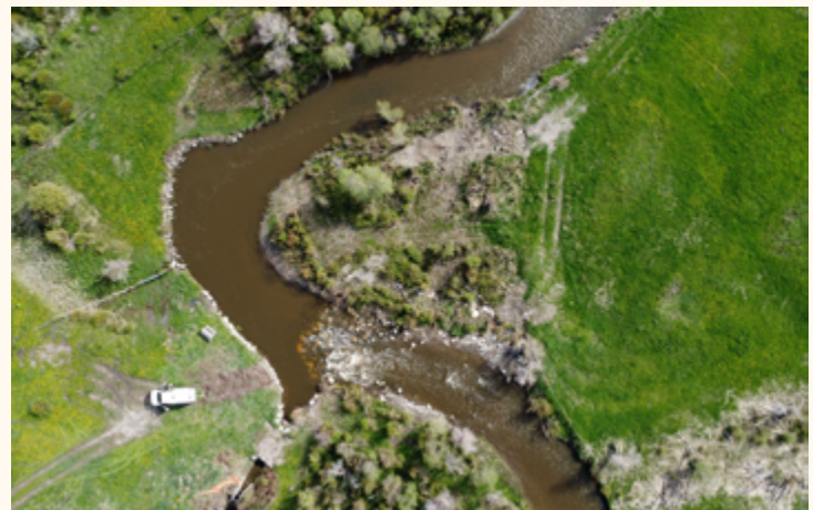
A diversion structure with an ecological rock ramp feature that allows for fish and sediment passage Photos and Project by Flywater, Inc.
