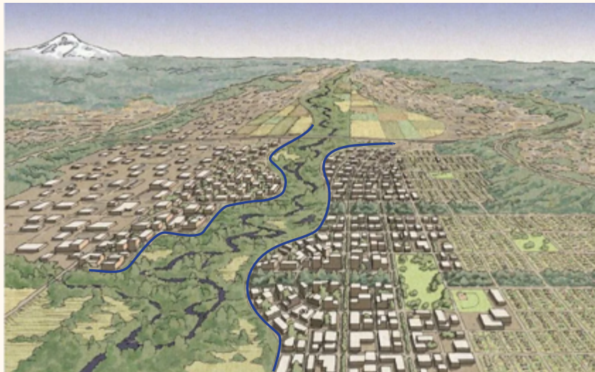
Setback levees (blue) allow room for a natural river corridor and an active floodplain | Illustration courtesy of Tony Melone
