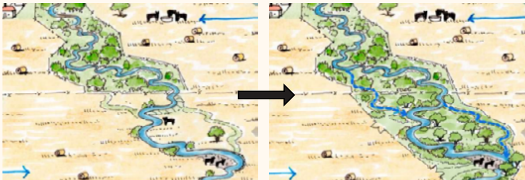
Side channels can be reconnected to reduce flood power and improve floodplain connection Drawings by Lauren Brown, LVBrown Studio
